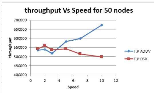
Fig28.THROUGHPUT VS SPEED FOR 50NODES
